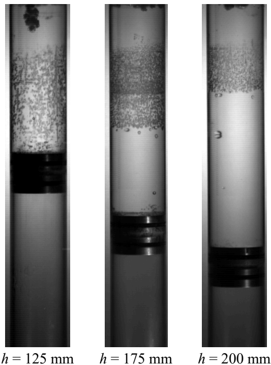
FIG. 15. Images of cavitation onset for typical experiments at different heights (multimedia available online). The experimental conditions are: (left) h = 125 mm, p_{t,max} = 4.0 MPa, and v_{p,max} = 10.1 m/s, (middle) h = 175 mm, p_{t,max} = 3.7 MPa, and v_{p,max} = 8.89 m/s, (right) h = 200 mm, p_{t,max} = 4.0 MPa, and v_{p,max} = 10.4 m/s.
