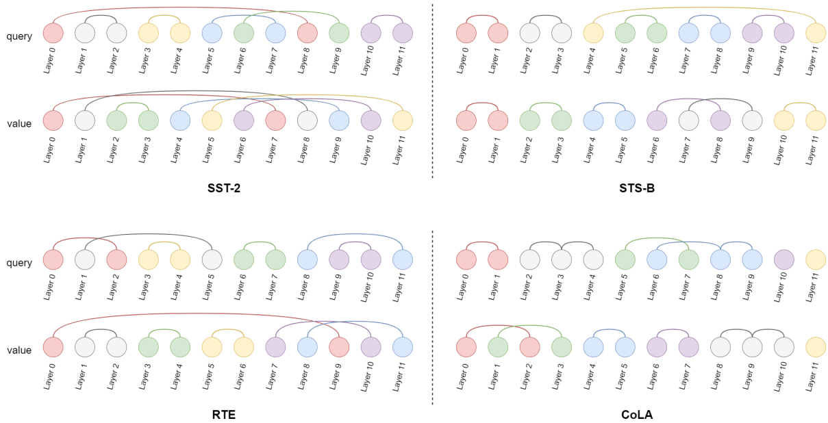
Figure 5: The allocation results of adaptive sharing on the GLUE Benchmark are presented. We set the merge times to 6 and report the sharing configurations of the query and value matrices. The same color represents sharing the same B matrix.
