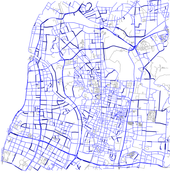
Fig. 10. Real-world road network of Nanjing (Partial). Blue lines refer to roads. Gray lines refer to unreachable roads or non-vehicle roads. Dark blue bold lines refer toroads with FCSs.
