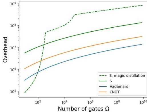
Figure 7: Overhead for the  $H$ , CNOT and  $S$  gates. The Hadamard gate using the lattice defect is now very cheap, while the overhead for the topological  $S$  gate has gained an order of magnitude over its counterpart using magic state distillation.
