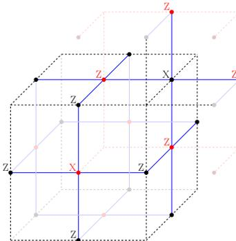
Figure 1: Unit cell of the 3D cluster states. The physical qubits are located on the red and black dots. The entanglement induced by the  $CZ$  gates is represented as a solid blue line.
