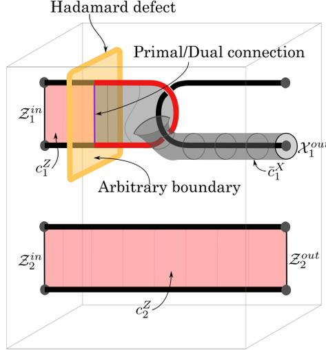
Figure 6: Hadamard defect and arbitrary virtual boundary connecting primal and dual surfaces. Thick black lines correspond to Z measurements on black qubits. Thick red lines to Z measurements on red qubits.
