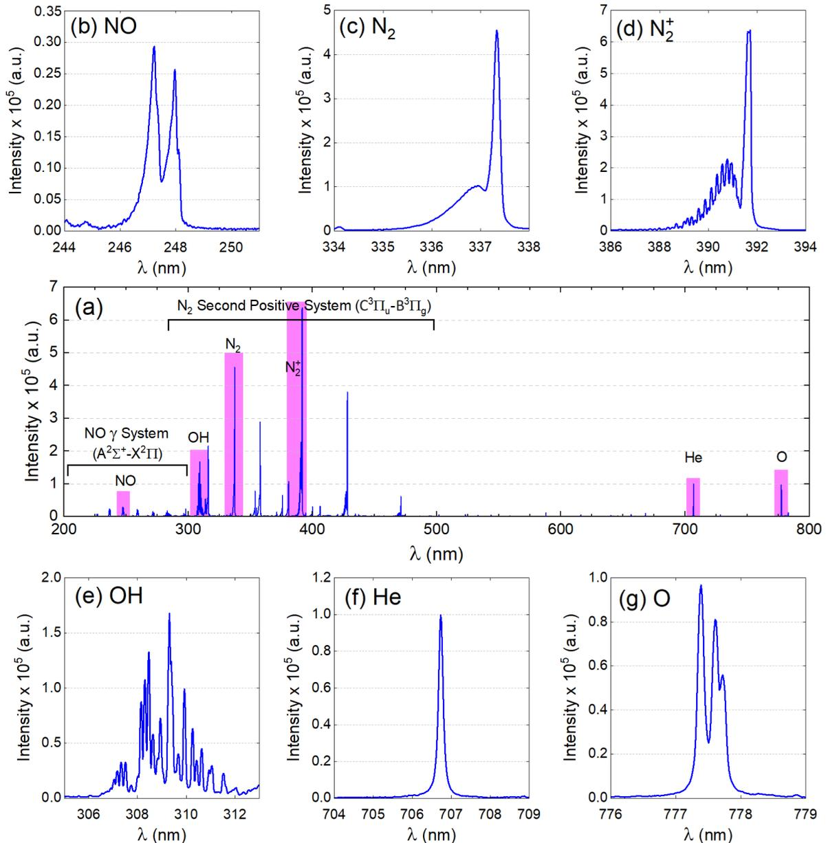
**Figure 3. Optical Emission Spectroscopy of the He-air plasma phase (a) Full spectrum from 200 to 800 nm, (b) NO\* radicals double-headed at 248.8 nm and 249.3 nm, (c) N<sub>2</sub>\* headed at 337.1 nm, (d) N<sub>2</sub><sup>+</sup> ions headed at 391.4 nm, (e) OH\* radicals at 308.9 nm, (f) He\* headed at 706.5 nm and (g) O\* radicals at 777.4 nm.**
