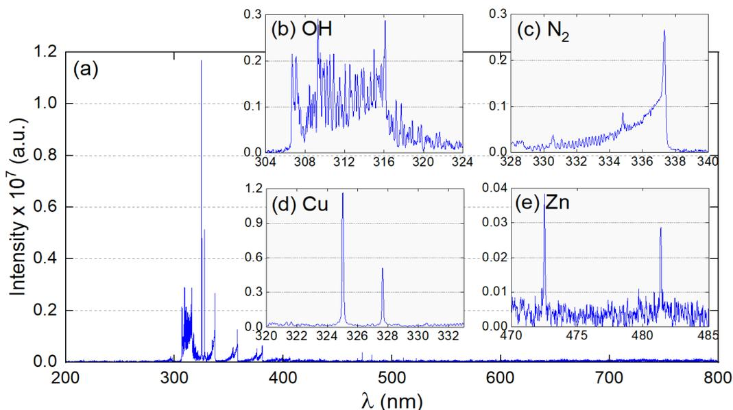
Figure 5. Optical Emission Spectroscopy of the plasma phase (a) Full spectrum from 200 to 800 nm, (b) OH\* radicals from 304 to 324 nm, (c) N<sub>2</sub>\* (C<sup>3</sup>Π<sub>u</sub>-B<sup>3</sup>Π<sub>g</sub>) headed at 337.1 nm, (d) Cu I (3d<sup>10</sup>4s-3d<sup>10</sup>4p) at 324.8 nm and 327.4 nm, (e) Zn I (3d<sup>10</sup>4s4p-3d<sup>10</sup>4s5s) at 472.2 nm and 481.1 nm.
