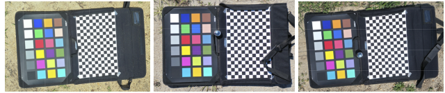
Figure 6. Images for photometric calibration. The drone imaging protocol includes images of the Macbeth card over multiple days. Although the same camera is used for imaging, camera parameters change. Notice slight variations in card appearance from different days, which we remove through photometric calibration.
