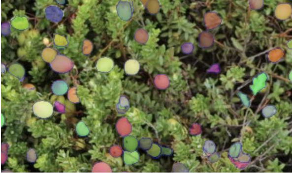
Figure 2. An example segmentation of cranberry images using the Segment Anything Model SAM [39] without point-click prompts (automatic mask generation). Notice that in addition to cranberries, surrounding leaves and other structures are segmented.
