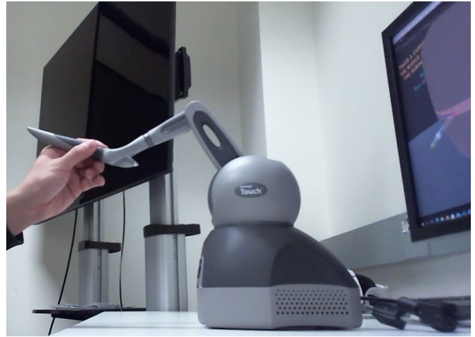
Fig. 4: A left-handed participant using the force-based haptic device for interacting with surface visualizations.
