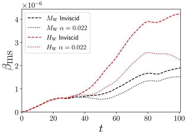
**Figure 11.** The mean-squared error  $\beta_{\text{ms}}$ , between the turbulent run tilt profile and that of the inviscid (dashed) or viscous (dotted) laminar runs. We compute this diagnostic for the ( $M_{\text{W}}, H_{\alpha}$ ) (black) and ( $H_{\text{W}}, H_{\alpha}$ ) (red) panels shown in Fig. 10.
