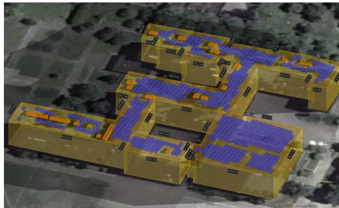
Figure 10. Modelling of solar energy system for the roof of Chortkiv Secondary School No. 5, taking into account some special features of the roof.
