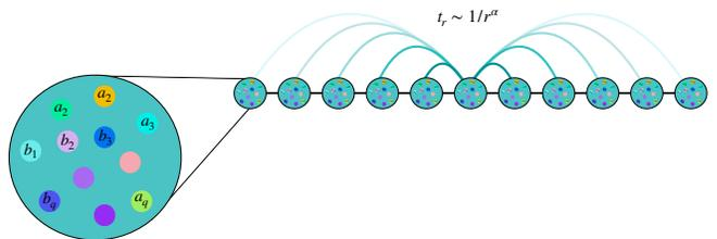
FIG. 2. Schematic representation of the  $\alpha$ -SYK model: a lattice of SYK dots connected through power law decaying hopping amplitudes.
