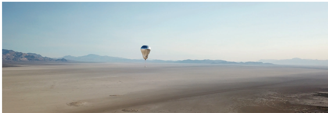
A subscale prototype of JPL's variable-altitude aerial robot, constructed from Venus-compatible materials, undergoing flight testing over the Black Rock desert in Nevada, USA in 2022. Credit: Aerostar/NASA JPL
