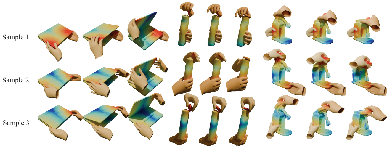
Figure 6. Diverse Results. We show diverse bimanual sequences together with the predicted contact maps on the laptop, ketchup, and mixer given the same unseen trajectory per object. Our method generates accurate finger placements guided by the predicted contact maps.
