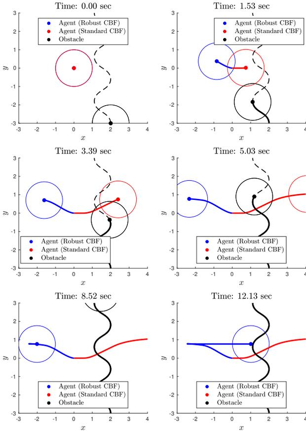
Fig. 1: System trajectory of agents in the presence of an obstacle (black) with unknown dynamics. The agent using the standard CBF (red) fails to avoid collision, while the agent considering the worst-case disturbance (blue) remains safe from the obstacle.
