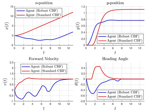
Fig. 2: System states of the agents representing the positional states  $[x(t), y(t)]$ , forward velocity  $v(t)$ , and the heading angle  $\theta(t)$ .
