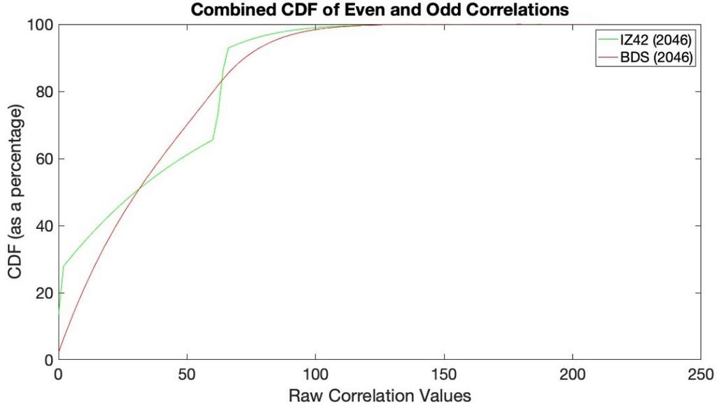
Figure 3: The figure plots the Cumulative Distribution Function (CDF) of all correlation values of the IZ4<sub>2</sub> and BDS B1 (truncated-Gold) spreading codes respectively. Values of the CDF are expressed as percentages.
