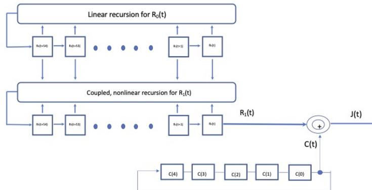
Figure 7: The IZ<sub>4</sub><sub>10</sub> spreading code can be generated using 2 55-bit binary shift registers and an additional 5-bit pure cycling shift register. The upper register is a linear feedback shift register. The lower register is updated using nonlinear logic using the contents of both shift registers.
