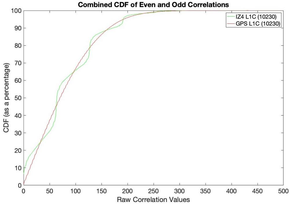
Figure 5: The figure plots the Cumulative Distribution Function (CDF) of all correlation values of the IZ4<sub>10</sub> and Weil spreading codes incorporated into ISRO’s NavIC L1 signal and the GPS L1 C pilot signal respectively. Values of the CDF are expressed as percentages. The maximum correlation magnitudes associated with the IZ4<sub>10</sub> and the Weil spreading codes are given by 484 and 500 respectively.
