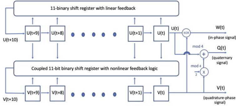
Figure 1: The  $IZ4_2$  spreading code can be generated using 2 11-bit binary shift registers. The upper register is a 7-tap linear feedback shift register. The lower register is updated using nonlinear logic using the contents of both shift registers. The figure also shows where to draw outputs corresponding to generating the in-phase  $\{W(t)\}$ , quadrature phase sequence  $\{V(t)\}$  as well as as composite quaternary spreading code  $\{Q(t)\}$ .
