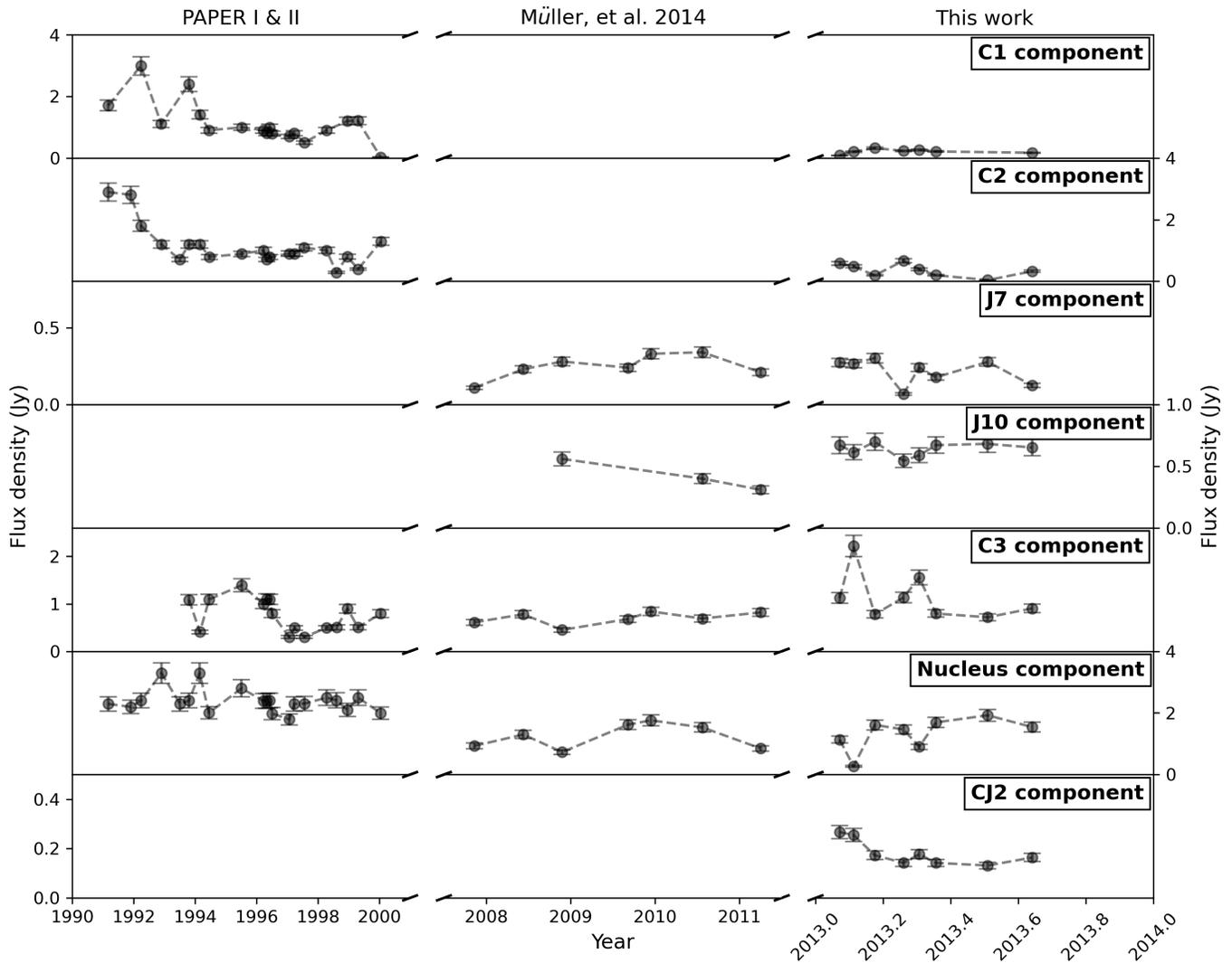
**Figure 5.** The light curves for all the model components. We also show the historical flux density evolution for the identified components from previous studies.
