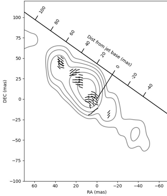
**Figure 10.** The Faraday rotation corrected intrinsic electric field directions in the subparsec scale jet of Centaurus A. In the background, we show the stacked 4.59 GHz image having applied the uv-range cutoff described in Section 3.2. As the diagonal axis, we show the angular distance downstream as measured from the jet base at 7.8 GHz. As the electric fields are measured from the epoch-stacked image, they represent the directions of long-term persistent fields in the jet.
