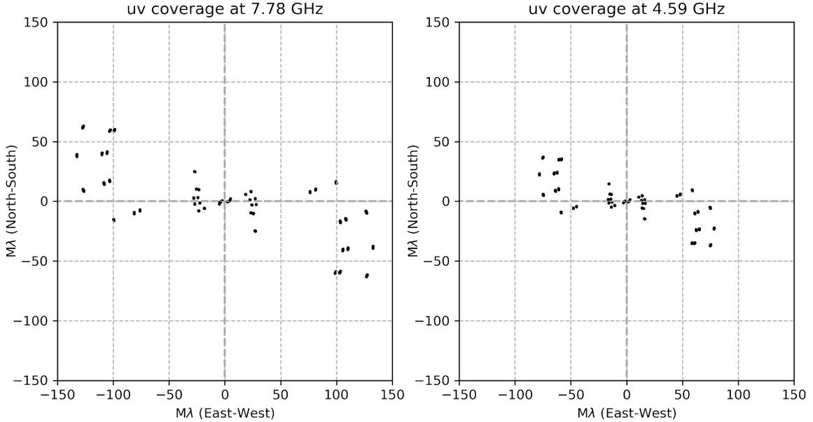
**Figure 2.** The uv-coverage at the highest and the lowest frequency bands for the epoch BO043A, after having flagged BR, HN, MK, and SC VLBA stations. The baseline lengths are measured in mega-wavelengths along the East-West and North-South directions.
