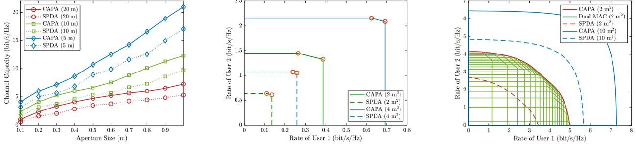
(a) Single-user capacity for different propagation distances (shown in the parenthesis). (b) Two-user MAC capacity region for different aperture sizes (shown in the parenthesis). (c) Two-user BC capacity region for different aperture sizes (shown in the parenthesis).
