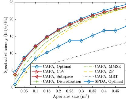
(c) Spectral efficiency achieved by different approaches in a downlink narrowband system with a uni-polarized CAPA transmitter and four uni-polarized single-antenna receivers, operating at 2.4 GHz. The impact of EM mutual coupling is omitted for the sake of brevity. Other simulation parameters can be found in [11].
