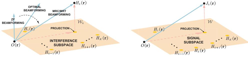
(a) Illustration of the heuristic beamforming design for CAPAs, where the MRC/MRT beamformer aligns with the user's spatial response, and the ZF beamformer is orthogonal to the interference subspace.
