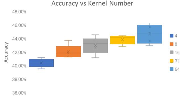
Fig. 5: Performance of Different Kernel Number Results show that the more kernel (TCN), the better performance.
