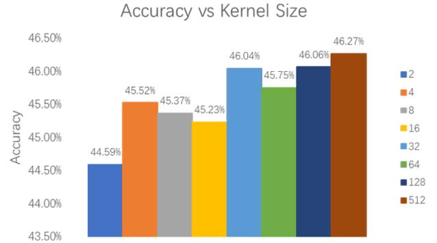
Fig. 6: Performance of Different Size of Kernel The size (length) of kernel has influence on performance. Finally 32 & 512 kernel size are selected, base on the performance.
