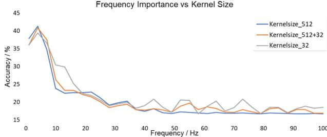
Fig. 7: **Frequency Importance of Different Kernel Size** Results show that model with big size of kernel such as 512, main focus on low frequency information, small size kernel like 32 can get information from relatively high frequency. However, when combine these two kernel size together, both low frequency and high frequency information can provide contribution, so this combination can use both low and high frequency information.
