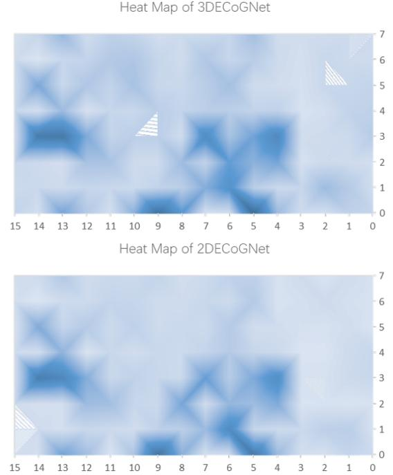
Fig. 9: **Heat Map for Each Channel of 3DECoGNet & 2DECoGNet** 128 channel reshaped to 8 x 16, which is same as electrode array, number of x y axis is used to define the position of electrode. Deeper color means bigger value which indicates more important for model performance. Results show that 3DECoGNet can extract more information from more channels, such as (10, 5), (6, 5), (2, 1)etc. compared with 2DECoGNet heat map,
