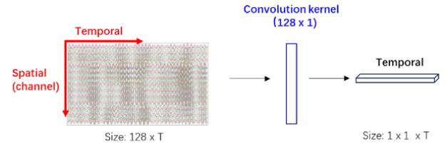
Fig. 8: **Spatial-Temporal Feature Encoder of 2DECoGNet** Each Spatial-Temporal feature map will processed by 1D convolution kernel, then get feature vector, the big difference compare with 3DECoGNet is that no reshape operation on the feature map.
