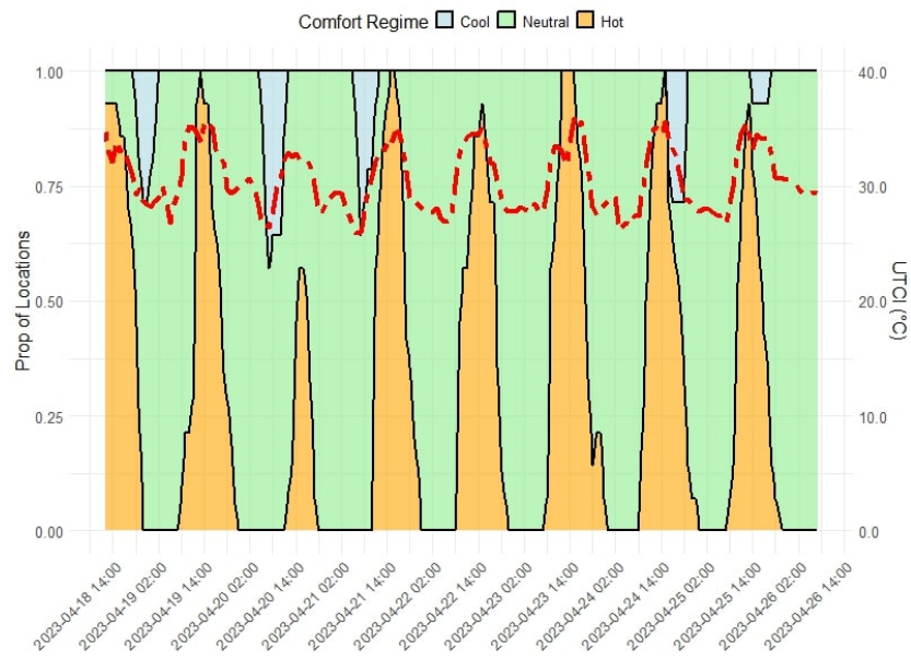
Figure 5: Temporal distribution of comfort regimes (Cool, Neutral, Hot) across locations, with the red dashed line representing the UTCI (°C) versus time. The left y-axis depicts the proportion of locations classified into each comfort regime, while the right y-axis indicates the UTCI.
