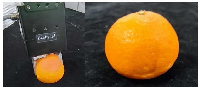
Fig 12. Irreversible damage to the deformable object, such as orange, irreversible dents emerge on the surface of the peel [96].
