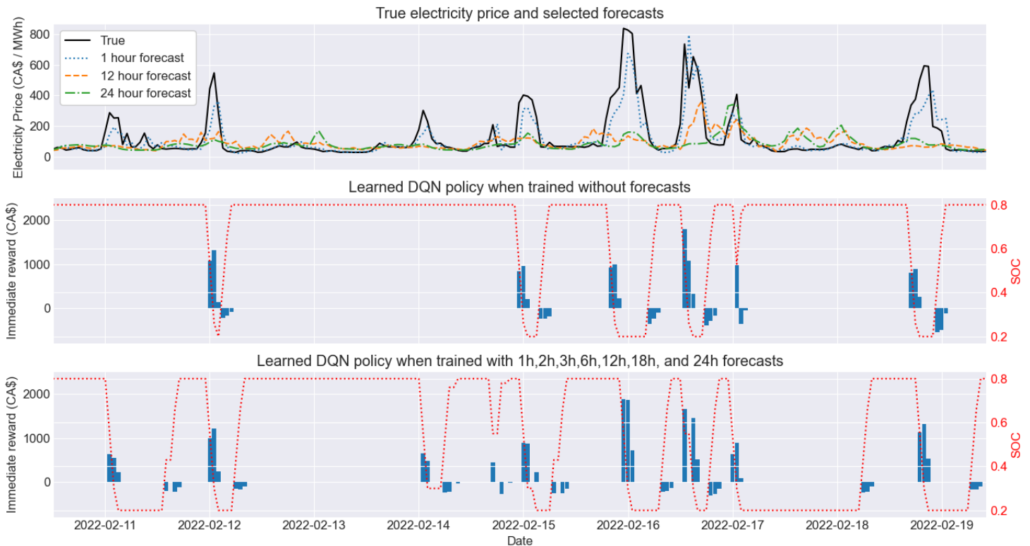
FIGURE 5: A nine day sample of (Top) true electricity prices and predictions for selected horizons with the best deep learning models found, (Middle) the battery SOC and rewards for a trained DQN agent without access to forecasts, (Bottom) for a trained DQN agent with access to all seven predictions.
