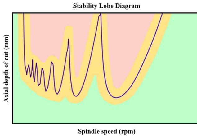
**Fig. 6.** Stability Lobe Diagram constructed considering the uncertainties inherent to their elements. The red, orange, and green zones depict the unconditionally unstable, conditionally stable (uncertain), and, unconditionally stable regions, respectively.
