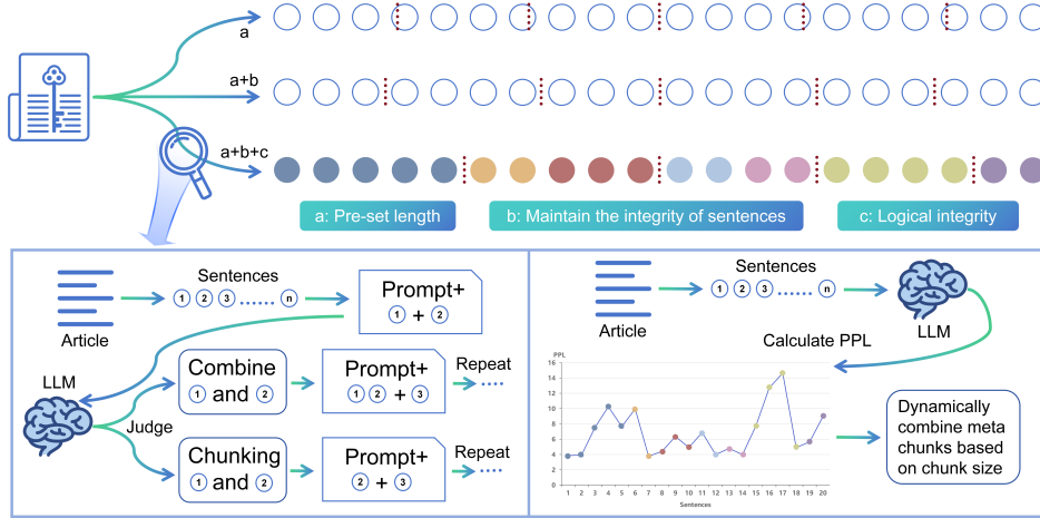
Figure 2: Overview of the entire process of Meta-Chunking. Each circle represents a complete sentence, and the sentence lengths are not consistent. The vertical lines indicate where to segment. The two sides at the bottom of the figure reveal Margin Sampling Chunking and Perplexity Chunking. Circles with the same background color represent a meta-chunk, which is dynamically combined to make the final chunk length meet user needs.
