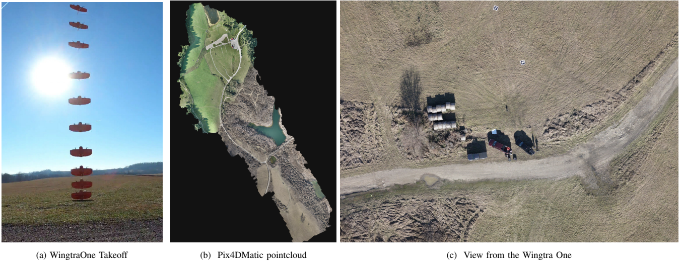
Fig. 4: The (a) WingtraOne 2 VTOL is used to collect images of the test site and produce a (b) high-resolution, geo-registered point cloud and mesh of the environment using the Pix4DMatic 3 photogrammetry software. (c) illustrates a view from the WingtraOne. This image is the test set up for the results shown in Fig. 11.
