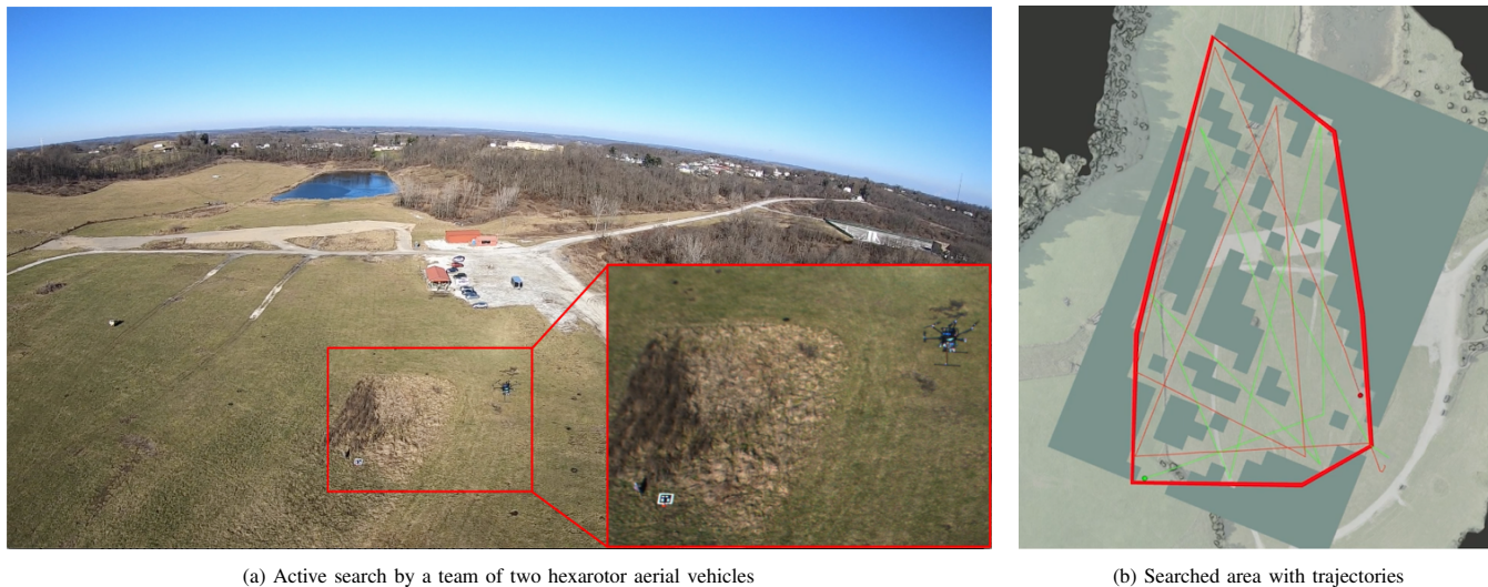
Fig. 1: Active search by a team of two aerial robots. (a) Image taken of one robot during flight. (b) The flight paths for each robot are shown in red and green plotted on top of a georegistered mesh. Unexplored cells are opaque and explored cells are transparent. The safe flight area is outlined in red. A video of this experiment may be found at https://youtu.be/lzh8M134enw . A video of active search conducted with three robots may be found at https://youtu.be/xgLnS2IFCQQ .
