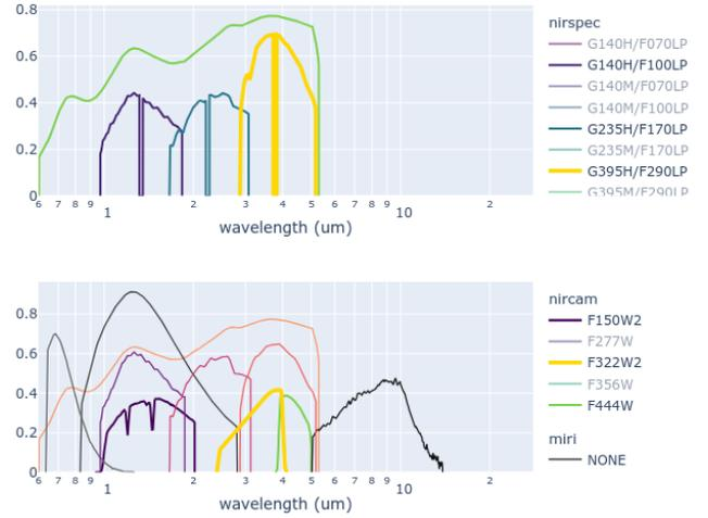
**Figure 2.** Filter throughput display for the NIRSpec instrument (top) or for all instruments (bottom). This display highlights the throughput currently selected (yellow thicker line) in addition to other available throughputs, helping the user to visualize the spectral range being covered and compare to that of other configurations. Users can interactively select/unselect which filters to display with the menu on the right hand side of the display.
