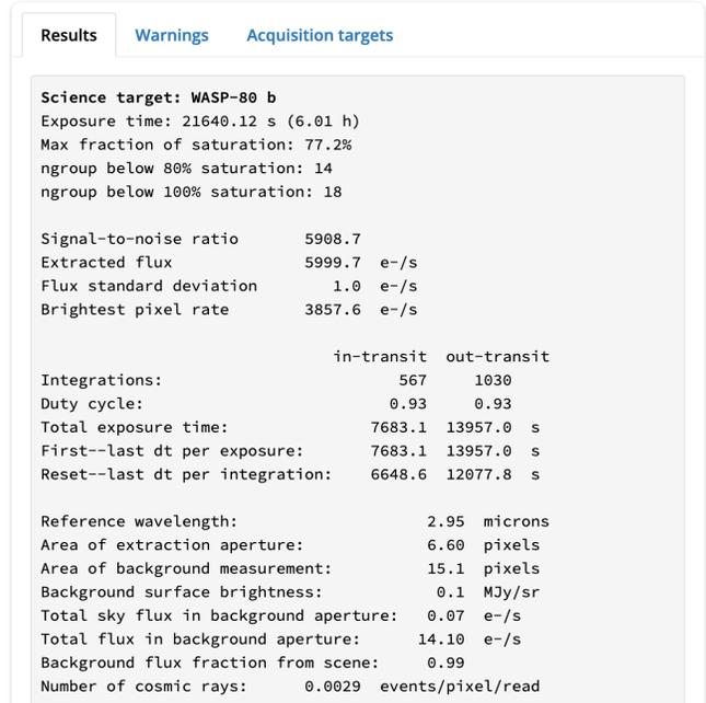
**Figure 6.** Results output text for a WASP-80b transit simulation with NIRSpec G395H/L290P.
