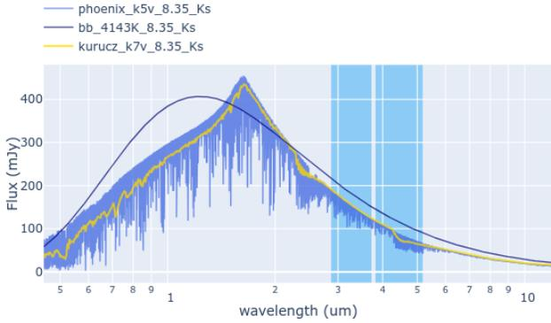
**Figure 4.** Stellar SED viewer panel of the GEN TSO graphical interface (Fig. 1). The solid curves show a PHOENIX (K5V, light blue), Kurucz (K7V, yellow), and a blackbody ( $T_{\text{eff}} = 4143$  K, yellow) SED models for the host star WASP-80. All models are normalized to a Ks magnitude of 8.351. The light-blue shaded area marks the spectral coverage of the filter currently selected in the application (NIRSpec G395H/F290P).
