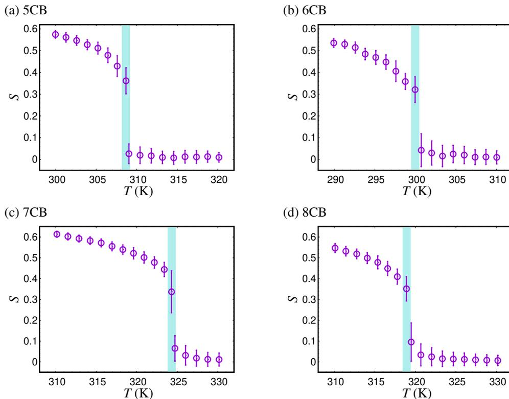
FIG. 1. Temperature dependence of orientational order parameter  $S$  for 5CB (a), 6CB (b), 7CB (c), and 8CB (d). The error bar at each temperature corresponds to the standard deviation. The vertical color bar indicates the NI transition temperature  $T_{NI}$ .
