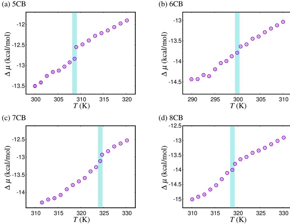
FIG. 4. Temperature dependence of the insertion free energy  $\Delta\mu$  for 5CB (a), 6CB (b), 7CB (c), and 8CB (d). The error bars at each temperature represent the standard deviation. The vertical color bar indicates the NI transition temperature  $T_{NI}$ .
