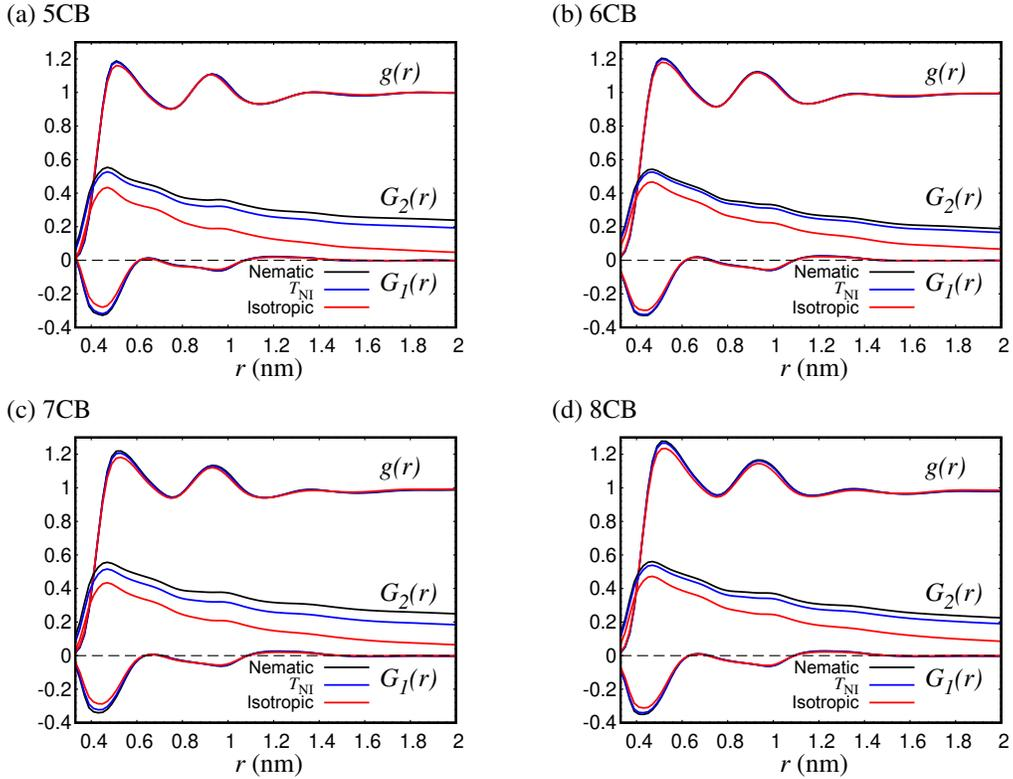
FIG. 3. Radial distribution function  $g(r)$  and orientational correlation functions  $G_1(r)$  and  $G_2(r)$  for 5CB (a), 6CB (b), 7CB (c), and 8CB (d). The results are plotted for replicas at  $T_{\text{NI}}$ , as well as for replicas above and below  $T_{\text{NI}}$  (isotropic and nematic phases).
