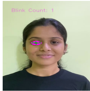
Fig. 3: Blink feature extraction by marking key eye landmarks and tracking blinking patterns.
