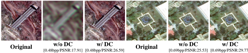
Figure 7: Contrast visual results. “w/ DC” means using of diffusion for compensation during decoding, while “w/o DC” indicates that diffusion compensation was not used during decoding.
