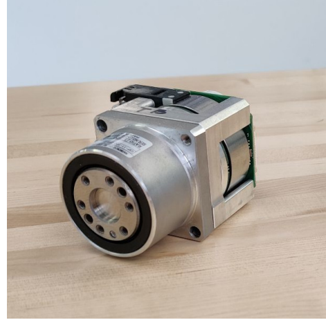
Fig. 3: Motor drive used to generate the training data, which consists of a motor with a Harmonic Drive gearbox. The gearbox introduces nonlinear oscillations into the system, leading to tracking errors at specific frequencies related to the input velocity. Photo courtesy of Alexandre Coulombe.
