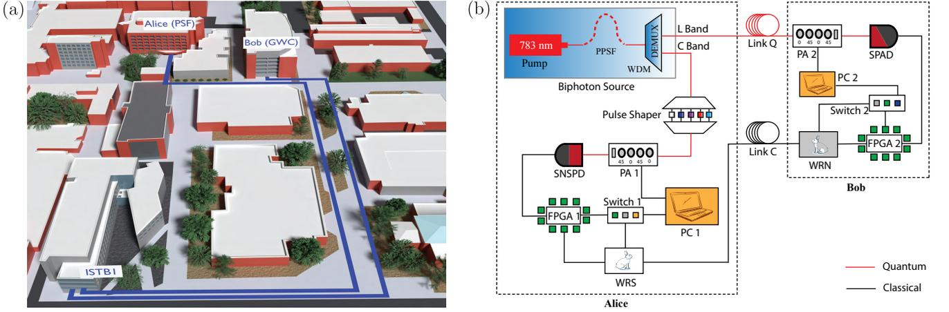
FIG. 1. (a) Map of the 1.6 km fiber link on the ASU campus. The blue line extending from Alice to Bob shows the fiber path. (b) Schematic of the overall setup including devices on both sides of the quantum link. Details are provided in the text.
