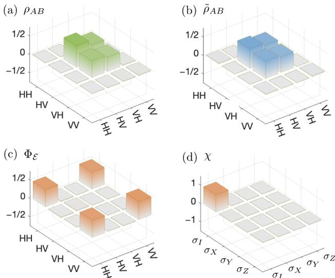
FIG. 2. Real parts of the inferred (a) input state  $\rho_{AB}$ , (b) output state  $\tilde{\rho}_{AB}$ , (c) Choi matrix  $\Phi_{\mathcal{E}}$ , and (d) process matrix  $\chi$ , where both  $\Phi_{\mathcal{E}}$  and  $\chi$  describe the dynamics of the quantum link. Local rotations have been applied to align reference frames, and all imaginary components (not shown) are less than 0.02.
