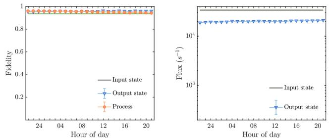
FIG. 3. (a) State fidelity of the output  $\tilde{\rho}_{AB}$  (blue triangles) and process fidelity of the link  $\Phi_{\mathcal{E}}$  (orange circles) over a 24 h period. (b) Detected photon pair flux of the output state (blue triangles) over the same 24 h period. The fidelity and flux corresponding to the input state are shown in green, with thickness denoting the Bayesian error bars.
