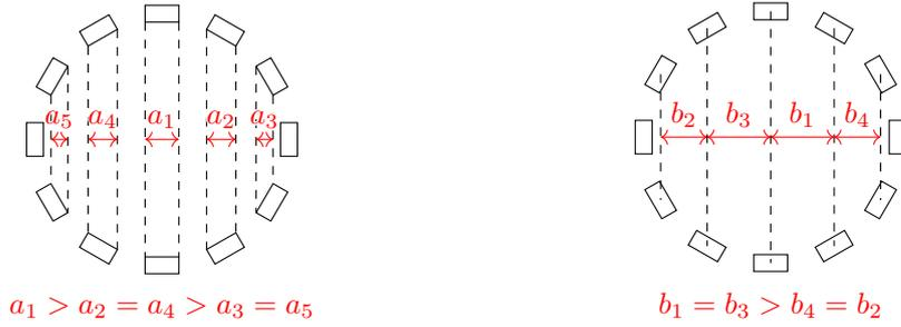
(a) Exposed detector width variation as a function of the radial position. (b) LOR distance variation as a function of the radial position.
