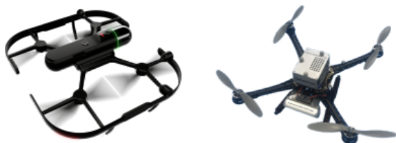
Fig. 7: MAVs used for real-world experiments. Left: Leica BLK2Fly with LiDAR. Right: Custom MAV with Intel Realsense D455 RGB-D camera.
