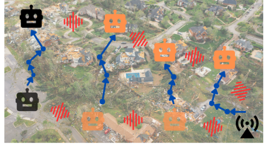
Figure 1: Illustration of a backbone reconfiguration with a different number of robots. The initial configuration is at the bottom, and the new one is shown at the top. The leader robot is depicted in black, and relay robots in orange. Planned trajectories (blue arrows), are guaranteed by construction to keep the backbone connected throughout the trajectories execution.
