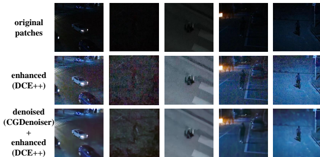
Fig. 7. Visualization of the denoising effect of CGDenoisier functioning on enhanced frames. Apparently, images after enhancement are seriously degraded by intricate real noise. With denoising support from CGDenoisier, the quality of frames recovers conspicuously.
