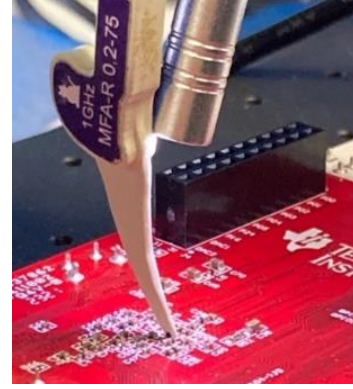
Fig. 1. The microprobe placed on the attacked board.
