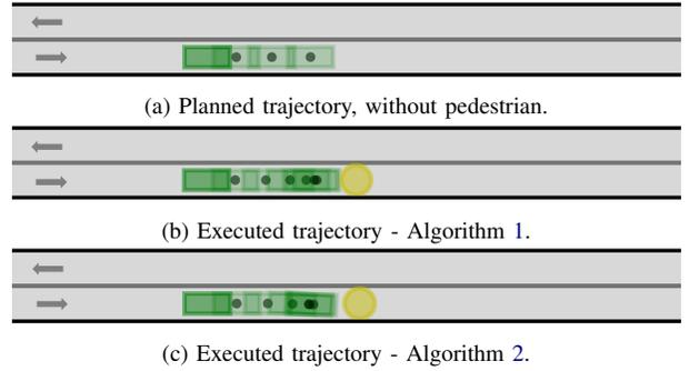
Fig. 3. Case study 1 - feasible scenario, initial velocity of  $18 \text{ km h}^{-1}$ . a) depicts the planned trajectory, b) and c) illustrate the executed trajectory once the jaywalker appears, using Algorithms 1 and 2 respectively.
