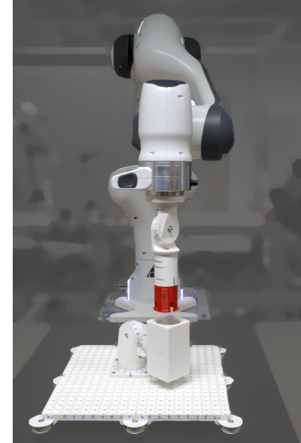
Fig. 1: POEMPEL task suite mounted on a Franka Emika 7-DoF robot arm. All parts are indexed and identifiable to ensure repeatability across attempts and labs. The red tip of the end-effector mounted plug is made from a flexible TPU material. The tip can be exchanged to others with different construction parameters, resulting in different stiffness levels and force requirements.
