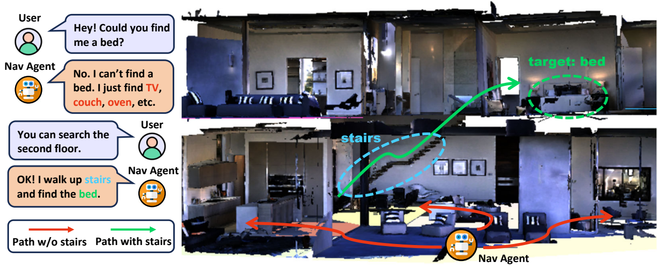
Fig. 1: The challenge of single-floor navigation. The target object of indoor object navigation is very likely to appear on different floors of the house, so the agent may not find the target object even if it has fully explored the current floor. Our proposed stair policy introduces the concept of indoor multi-floor navigation and proposes a feasible and learning-free solution to this challenge.
