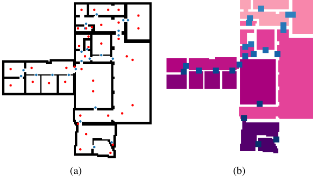
Fig. 3. (a) Obtained poses of rooms and doors. The red point represent the poses of rooms. The blue points represent the poses of doors. (b) Created segmentation of the scene. The red and blue areas represent different rooms and doors respectively.
