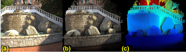
Fig. 5. A sample output from our mapping evaluation algorithm. (a) displays the original image captured by the camera. (b) shows the image as rendered by our algorithm, and (c) presents the depth map, derived from the point cloud, which was used in the rendering of image (b). The rendered image (b) is then compared to the original (a) for evaluation using metrics such as Peak Signal-to-Noise Ratio (PSNR) and Structural Similarity Index Measure (SSIM).
