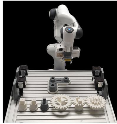
Fig. 2: Experiment setup with a franka panda robot, four toolcubes from Leverage, and a gearset from the Siemens Robot Assembly Challenge
