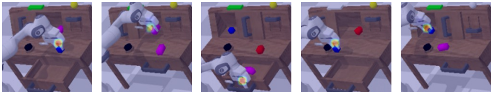
Figure 14: Visualization on attention maps of the policy model. The policy model demonstrates the ability to direct attention towards the end-effector and the object it interacts with, without the need for explicit supervision during the learning process.
