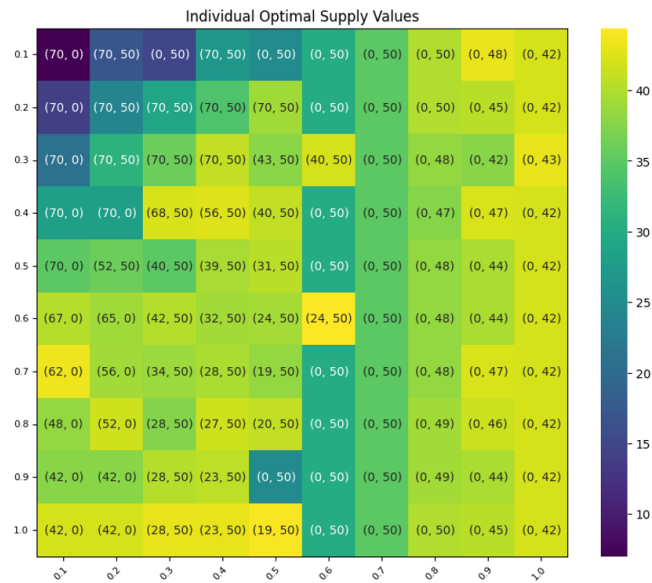
FIG. 12. Optimal Supply Quantities: This heat map shows us how much units of the part to order from the suppliers, based on their reliability using QMC. Heatmap showing the model’s preference shift from supplier 1 to supplier 2 as supplier 2’s reliability increases, despite the latter’s lower cost. The x -axis corresponds to the reliability of the second supplier, while the y -axis corresponds to the reliability of the first supplier.
