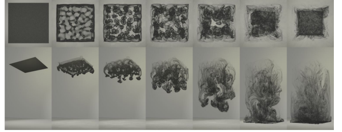
Fig. 14. RT Instability. The initially thin layer of ink at the top of the water tank gradually becomes unstable. Through the process of coalescence, it forms many small ink drops. These aggregated ink drops begin to fall and take on the classic figure shape of RT instability.
