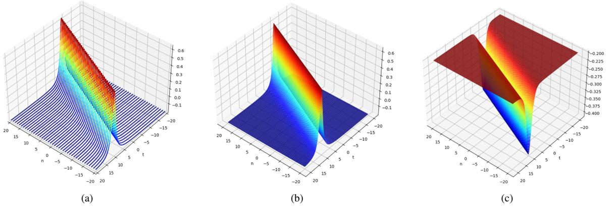
**Fig. 1:** Shape and motion of first order solutions ( $Q_n$  is presented) for the focusing sd-mKdV equation. (a) and (b) A soliton with  $a_0 = 0.2$ ,  $k_1 = 0.2$ ,  $c_1 = -d_1 = 1$ . (c) An anti-soliton for  $a_0 = 0.2$ ,  $k_1 = 0.3$ ,  $c_1 = d_1 = 1$ .
