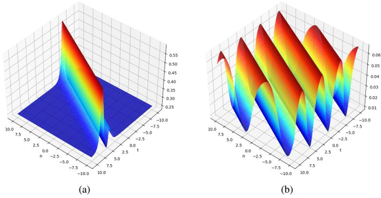
**Fig. 6:** Shape and motion of first order solutions ( $|Q_n|^2$  is presented) for the defocusing reverse-space-time sd-mKdV equation. (a) Soliton with  $a_0 = 0.5$ ,  $k_1 = 0.2j$ ,  $c_1 = -d_1 = 1$ . (b) Doubly periodic wave with  $a_0 = 0.1$ ,  $k_1 = 0.3j$ ,  $c_1 = -d_1 = 1$ .
