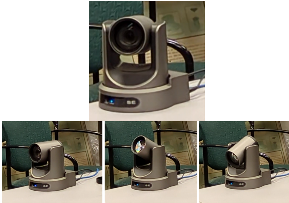
Fig. 2. (Top) The ImproVision robot turns to make pseudo “eye contact” with the violinist. After turning to indicate who ImproVision is communicating to, it will then provide an instruction through its motion. (Bottom) The process of providing an ensemble down-beat: the ImproVision robot first looks to ensemble center, lifts, then bows its head.
