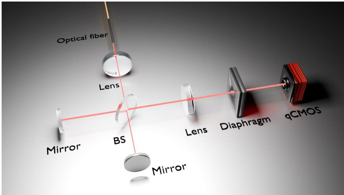
**Fig. S2** Experimental setup for coherence measurements.
