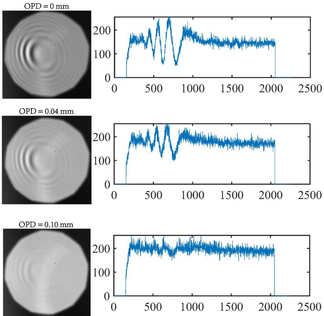
**Fig. S5 Determination of coherence length.** Left: Coherent fringe image (OPD = 0 mm, 0.04 mm, 0.10 mm) taken by the camera. Right: Intensity distribution on the central transverse line of the corresponding image after MATLAB processing.
