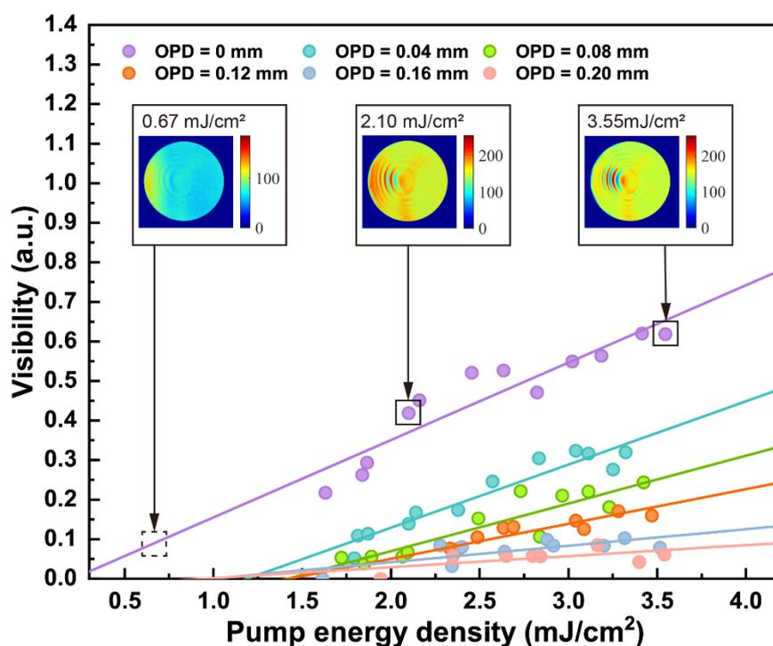
**Fig. 3** The dependence of the fringe visibility on the pump energy density under different OPDs. The correlation between the fringe visibility and the pump energy density is indicated by the linear fitting. Inset: the fringe patterns collected under different pump energy densities at zero OPD. The dashed box denotes the low visibility of the fringe obtained with the pump energy density far below the lasing threshold.
