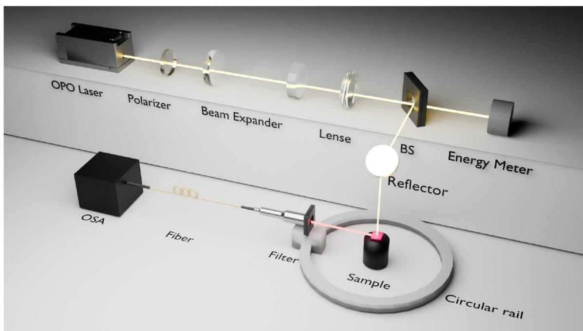
**Fig. S1 Experimental setup for Lasing and directivity measurements.** The Filter and fiber port are fixed on a movable platform that slides freely on a circular rail. OSA: Optical Spectrum Analyzer.
