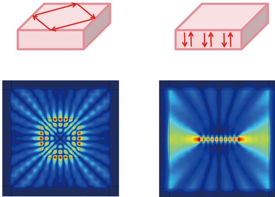
**Fig. S3** Laser mode schematic and diagram. Left: Whispering gallery mode formed by four sides. Right: Fabry–Pérot mode composed of upper and lower planes.
