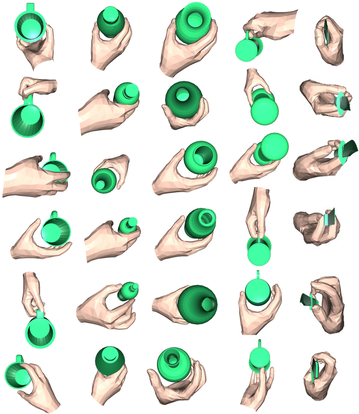
Figure 6. Given a single object, our method is capable of generating different grasps on it.
