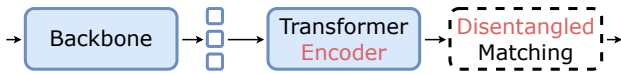
Figure 4: Comparison with existing transformer-based 3D object detection methods. We introduce encoder-only transformer architecture w/o positional encoding for queries or attention layers. This allows us to change unstable Hungarian matching for a simpler disentangled scheme.
