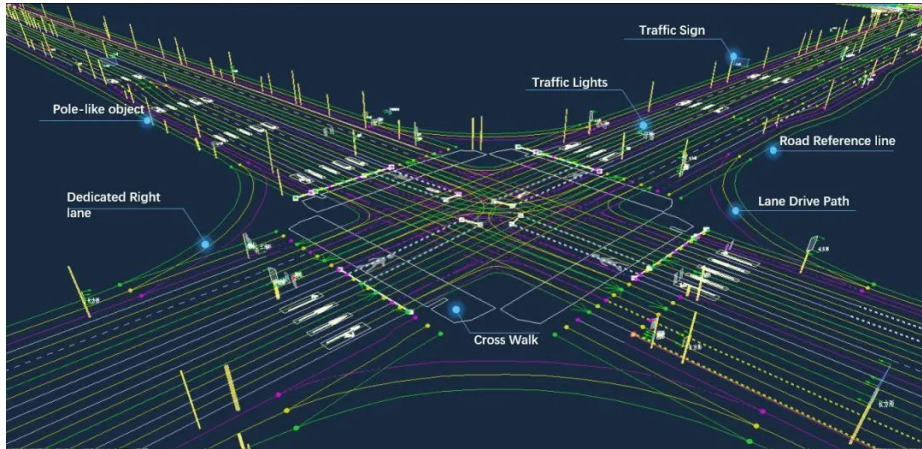
Fig. 1. Illustration of a snapshot of vectorized HD map. It is composed of static map elements, such as pedestrian crossings, lane dividers, road boundaries, etc., which are geometrically discretized into polylines or polygons.
