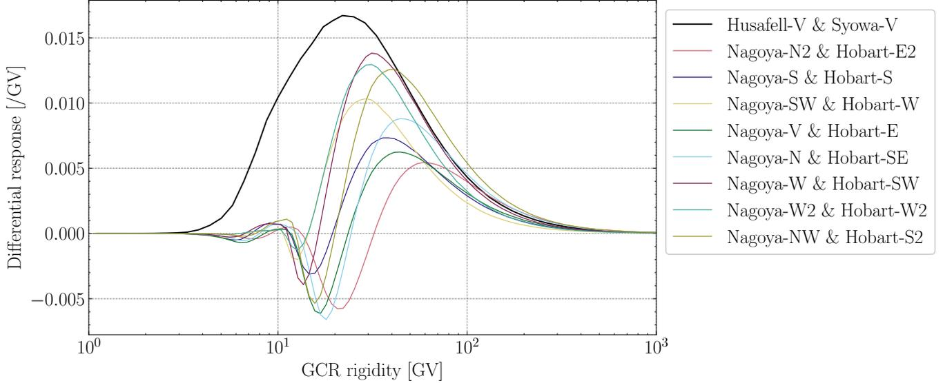
**Figure 7.** Black bold line is a differential response to the NS anisotropy for vertical channels of muon detectors at Husafell, Iceland (virtual detector) and Syowa Station. Other solid lines are repeats of those in Figure 2.
