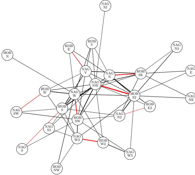
**Figure 1.** Visualization of general graph matching for optimizing channel pairs. Each node corresponds to a directional channel, and each edge connecting the nodes represents each channel pair. The line width of each edge is proportional to the sensitivity  $a_{ij}$  of each pair  $ij$ , and red edges represent the pairs derived as the optimal solution.
