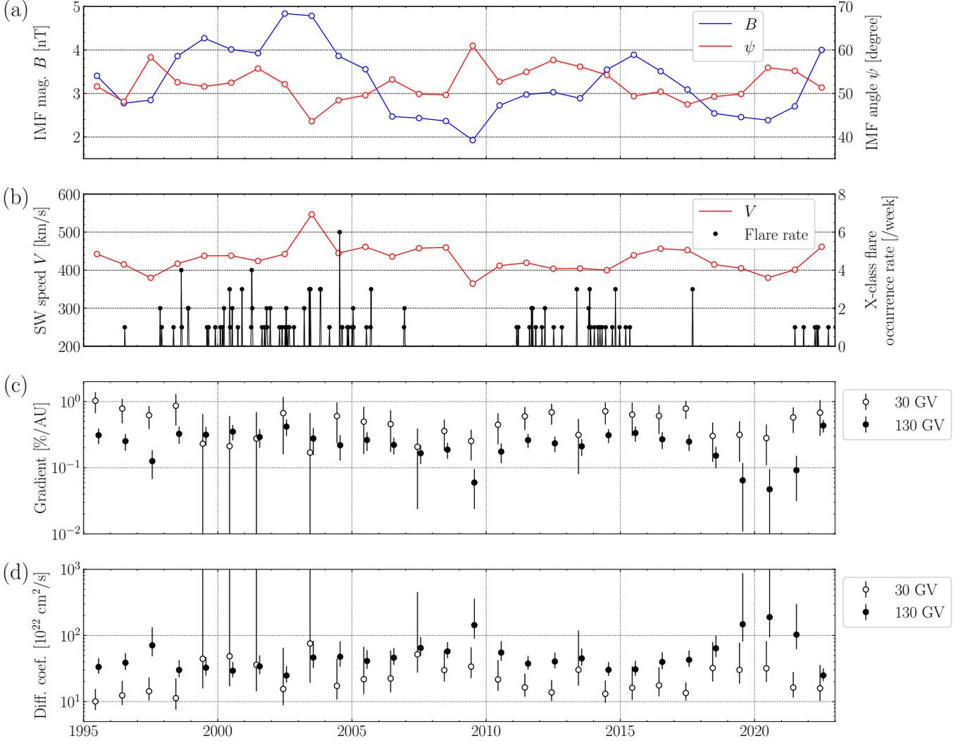
**Figure 5.** Temporal variations of the solar activity, interplanetary, and GCR modulation parameters. (a) Yearly averages of the magnitude  $B$  [nT] and spiral angle  $\psi$  of the IMF. (b) Solar wind (SW) speed  $V$  [km/s] for each year and X-class flare occurrence rate every week. (c) Radial density gradients [%/AU] and (d) diffusion coefficients [ $10^{22}$  cm<sup>2</sup>/s] of (open circles)  $\sim 30$  GV and (solid circles)  $\sim 130$  GV GCRs derived from the yearly NS anisotropy.
